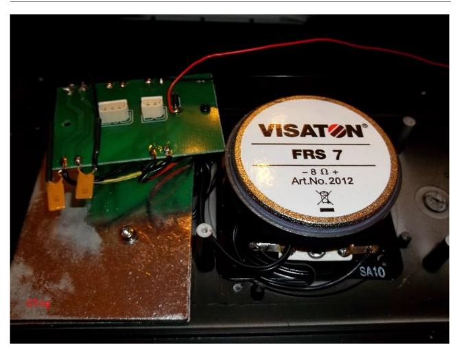
Remove the cable at the rear. Remove the PCB. Remove the front weights. Add 2 pole cable additionaly to the 4 others to the front. Solder the cables as shown. To do this remove the bogie. With an original bracket of the speaker you can fix the cables. Solder the speaker cable from speaker to Stocko pin connector socket.
