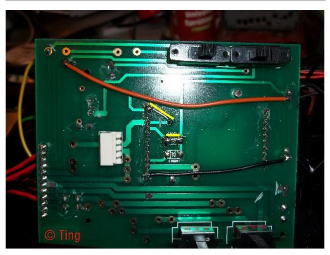
On the top side remove parts marked with X and cut off 3 conductor tracks. Approximately at the position marked with arrows put the XXL decoder as drilling jig and draw the holes on the PCB. Make sure that you drill no conductor track!
