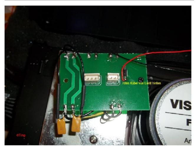
Before you screw on the loco, test all functions! Put the loco and tender on the track, connect the 6 pole stocko plug.
