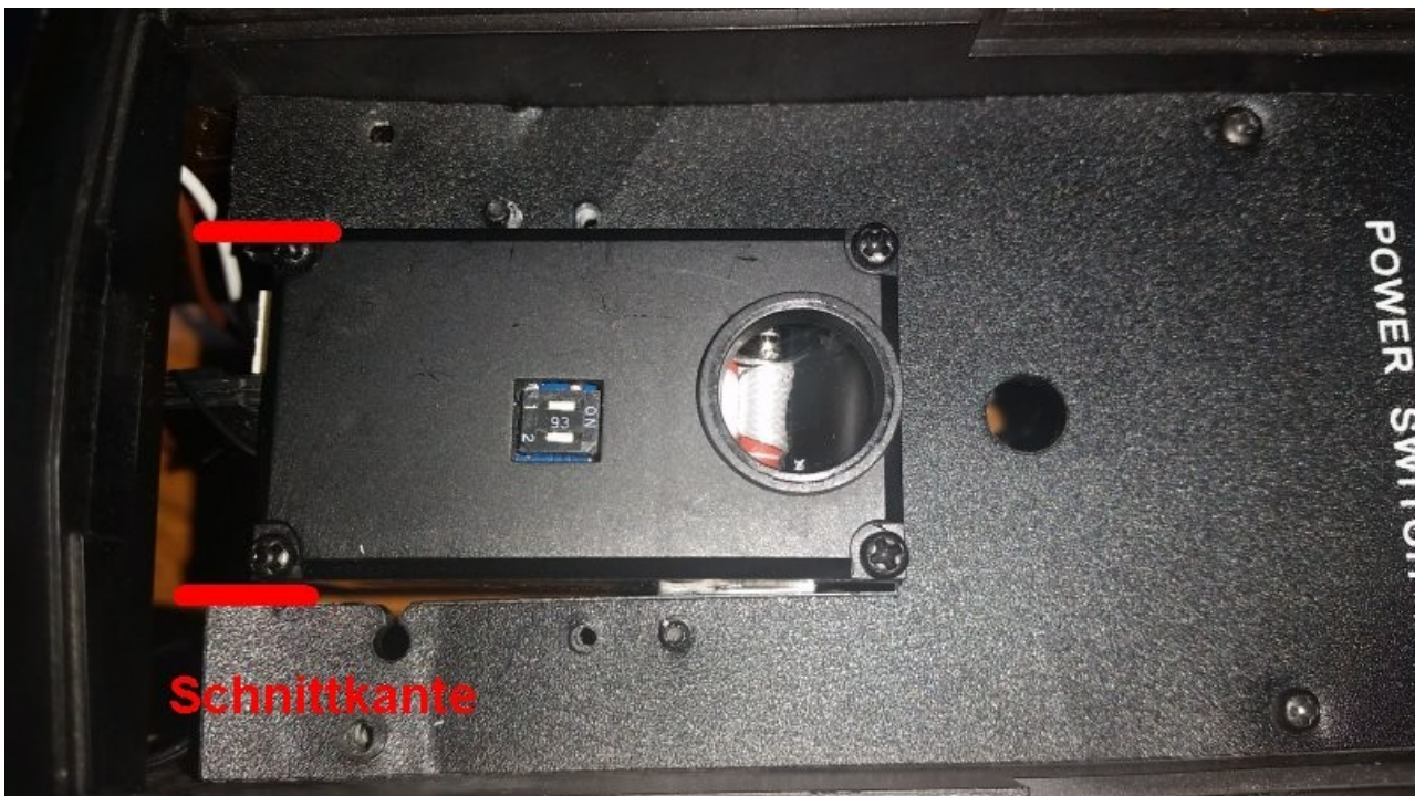
Figure-4: Modification of the PCB mounting board
