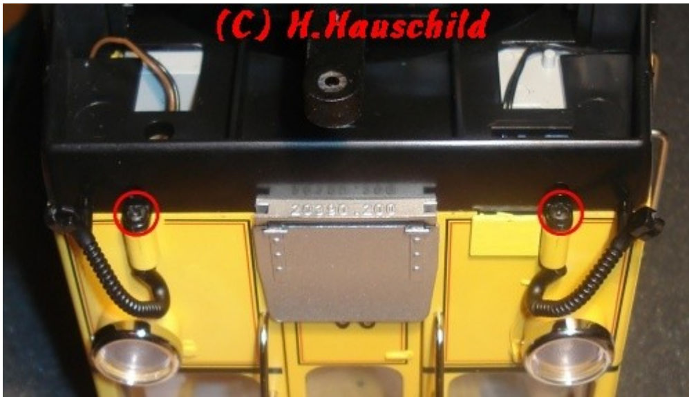
Pict.-2: Screws under break hoses
