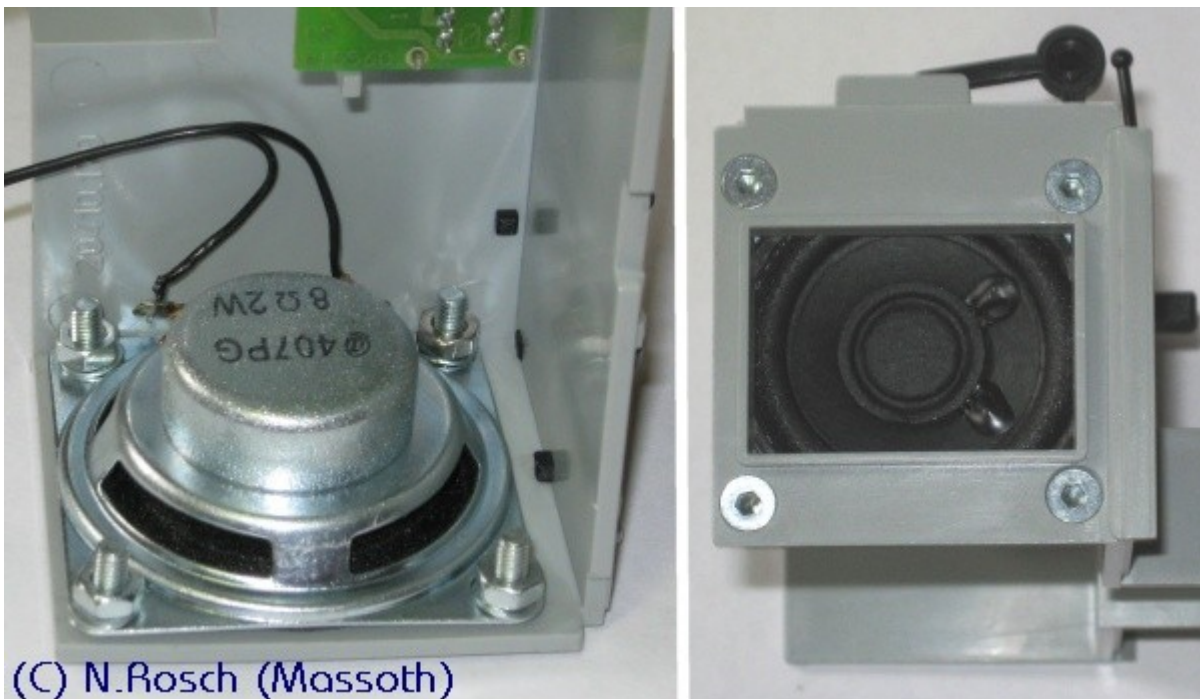
Pict-3: Installing speaker
