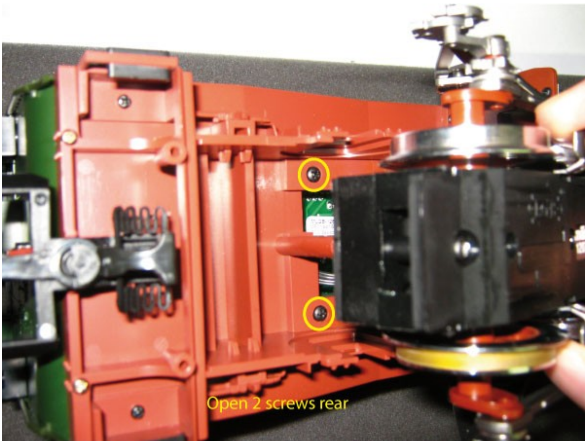
Figure-2: Removing the rear 2 screws under the gear.
