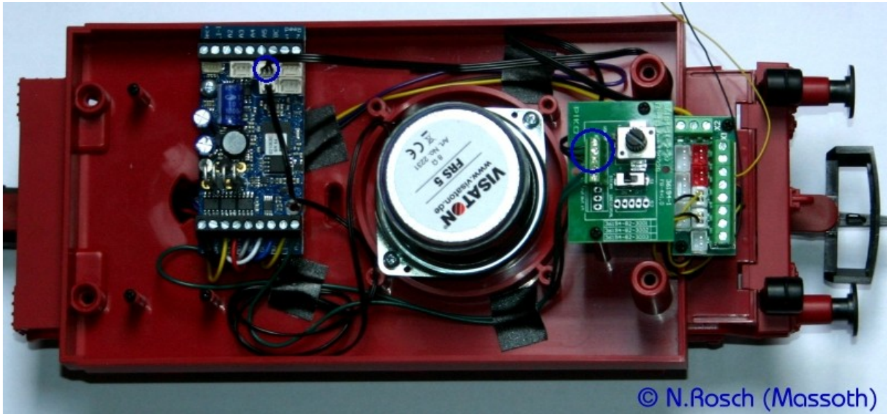
Picture 4 : Mounting of the decoder and speaker
