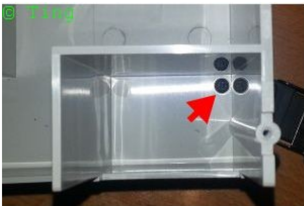
Pict 6-9: Open the screws for inner part.
