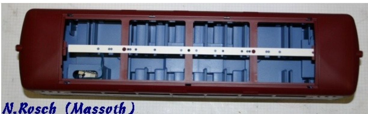
Picture-8: Light strip installation
