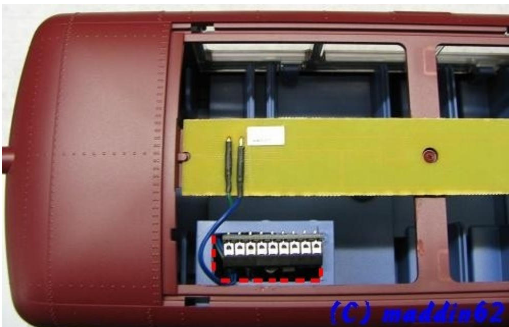
Pict.-5: Assembling decoder in the toilet and assembling the roof illumination.
