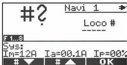
The selected locomotive may now already be operated with the dial knob. A simple driving operation is available. The locomotive is operated with 28 speed steps and parallel functions.
