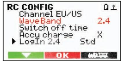
Only the 2.4 GHz frequency band can be used with the permanently integrated 2.4 GHz radio chip. The firmware also supports the EU/US frequency bands, but these have no effect here. A selection of the wrong frequency bands only leads to a shutdown of the radio system (see also chapter **LogIn 2.4GHz**).
