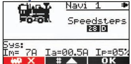
Holding **M2** long (three seconds) will load the loco configuration mode. The first configuration page provides a function to delete locos that are not required anymore. Holding **M1** will delete the active loco from the Navigator. Afterwards a new loco can be selected with **M1** and **M2** and confirmed with **M3**.
