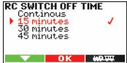
The radio shutdown time (standby time) determines the duration of the operating time when the Navigator is not in use until it automatically logs off and switches off. In the event of switch-off or loss of reception, all assigned locomotives are automatically logged off.
