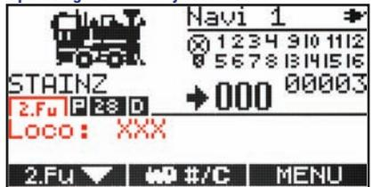
The DiMAX Navigator can operate two different locomotives at the same time independently. The second locomotive is controlled with the secondary function keys and is performed as follows:
