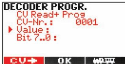
CV Programming is the most common way of programming nowadays. It is supported by most of the available DCC systems. It required entering the CV and programming value followed by **M2**. Depending on the DCC system the programming procedure is performed on a separate programming track or the main track used as a programming track (Please check your central station manual for further details).
