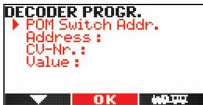
With this feature the latest state-of-art switch decoders may be programmed. **When entering the address, the “M1” key can be used to switch between decoders with standard and extended switching commands (eS).** Please refer to the manual in
