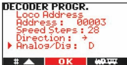
The loco address can be read and programmed with this menu. The address may be selected within the range from 1-10239. Depending on the number of speed steps, driving direction and analog functionality, the Navigator will automatically calculate the programming values for CV 1, 17, 18 and 29.
