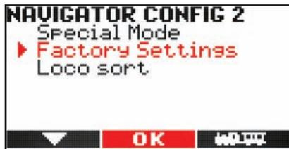
Confirm the factory reset of the Navigator only when you are absolutely sure. If not please leave the menu with **M3**. If the factory reset is executed all configurations will be deleted. Afterwards the Navigator starts with factory settings. All configurations need to be entered again (locos, switching routes, double heading, switches,...).
