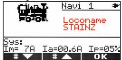
Define your personal loco name which is displayed below the locomotive picture in the driving mode. The loco name is also displayed when a locomotive is operated in the secondary function layer. The loco name is shown below the loco address. Press **M1** and **M2** or rotate the wheel knob slowly to browse through the list of available
