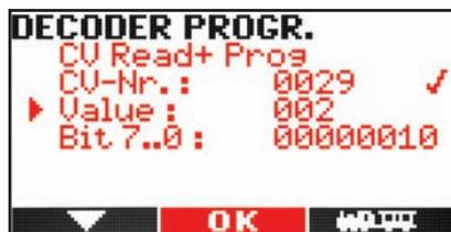
Some CV's consist of several binary values. This gives the opportunity to configure several settings within one CV. Every function has one single bit location (like a switch) and a value. If such a CV needs to be programmed, all values of active bits need to be added up. A deactivated function has always the value 0,
