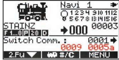
When special mode 3 is activated, the feedback data of triggered track contacts connected to feedback modules are shown in the display of the Navigator. When the switch command function is selected for the secondary function display the feedback details are shown below the switch address. The first four digits show the triggered contact address as it is used for PC control, the last 5 digits show the programmed contact number.
