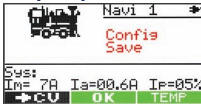
Prior saving the loco configuration itself it is possible to save the configured details into the decoder. The loco needs to be placed on the programming track of the central station (CV programming). **M1** will start the programming procedure.
