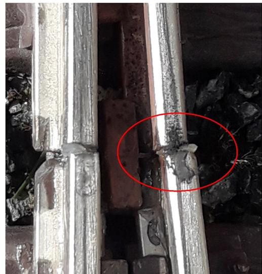
The image on the right shows a close-up of two insulation points on a switch where proper insulation is no longer guaranteed. The insulating plastic has worn away or disappeared entirely. This results in unwanted short circuits and feedback from the incorrect rail side into the EVO-X, which can lead to the aforementioned damage. The burn marks visible on the track are further evidence of this issue.
