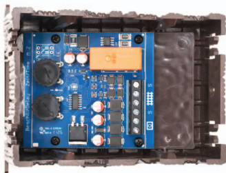
Abbildung 2: Einbau der Pendelautomatik in LGB Prellbock Nr. 10310 Illustration #2: Fitting the Automatic Shuttle in LGB bumper no. 10310
